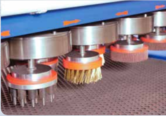
Tool options for WEBER P2 / P6 for deburring, descaling and rounding.
